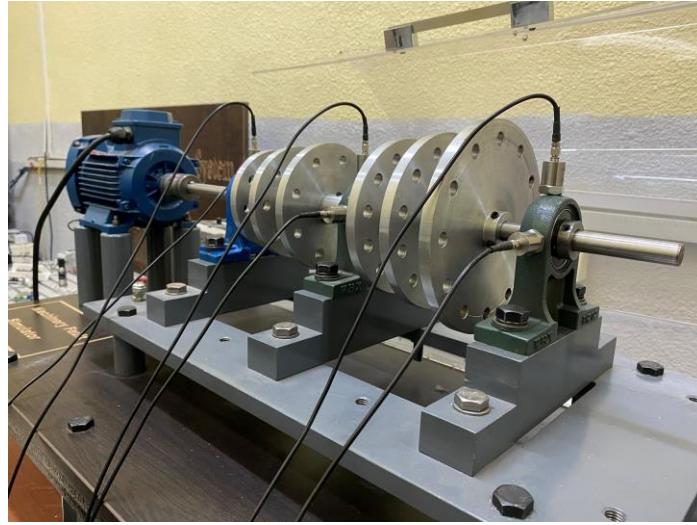
Figure 1. The design of the rotating machine simulator
