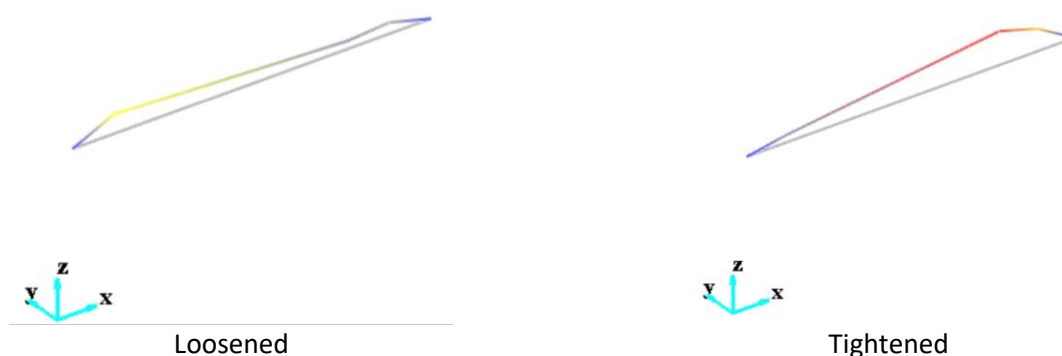
Figure 5. First mode shapes in two different types of OMA test
