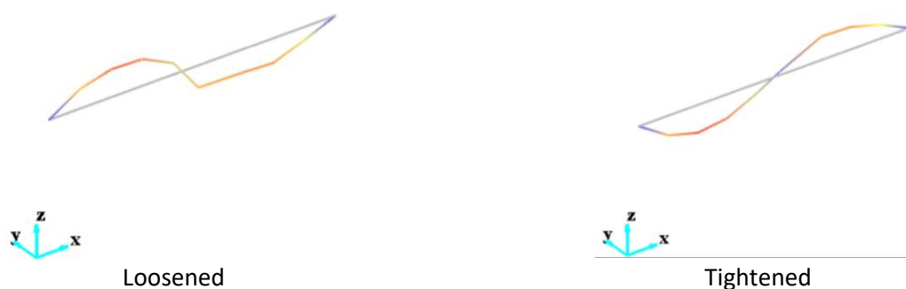
Figure 4. Second mode shapes in two different types of EMA test
