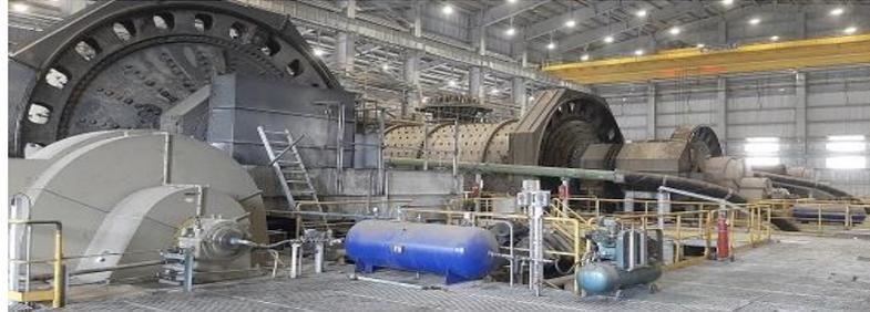
**Figure 2.** Overflow ballmill.
