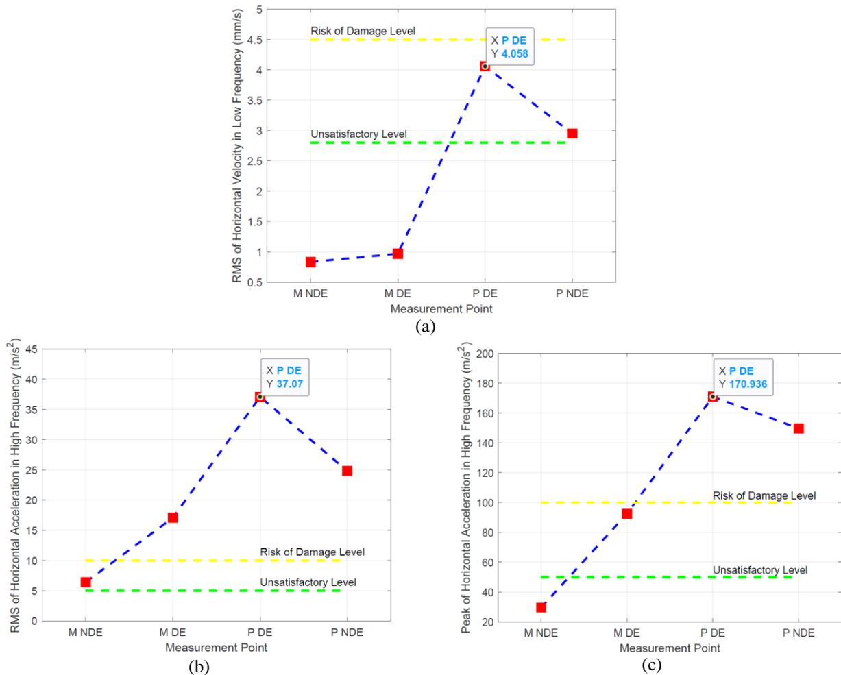
**Figure 3.** Change in vibration parameters over measurement points in horizontal direction: (a) RMS of velocity in low frequency, (b) RMS of acceleration in high frequency, (c) Peak of acceleration in high frequency.
