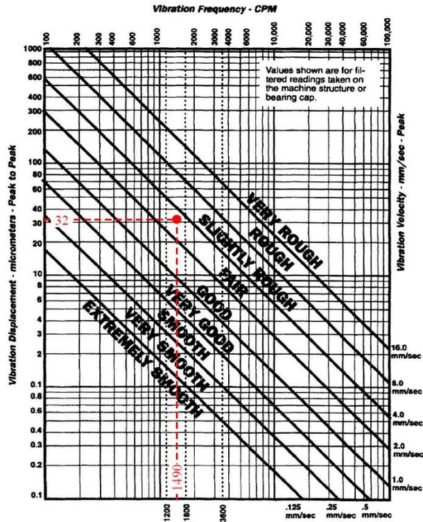
Figure 2. ENTEK IRD general machinery vibration severity chart.
