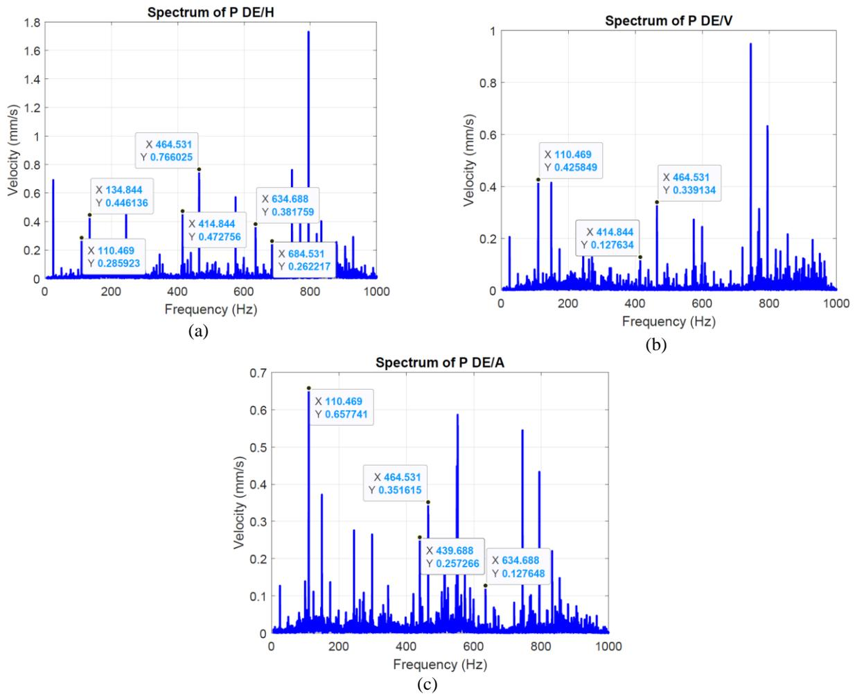
**Figure 4.** Spectrums of “P DE” measurement point in: (a) Horizontal, (b) Vertical, (c) Axial directions.
