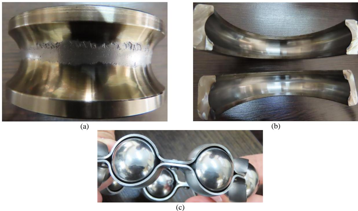
**Figure 5.** Real images from different components of “P DE” bearing: (a) Inner race, (b) Outer race, (c) rolling elements.
