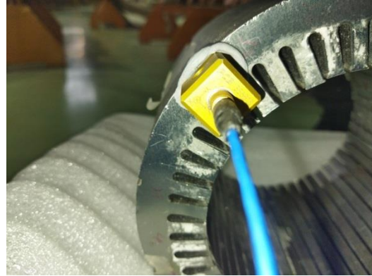
Figure 3. Sensor installation point and its axes directions
